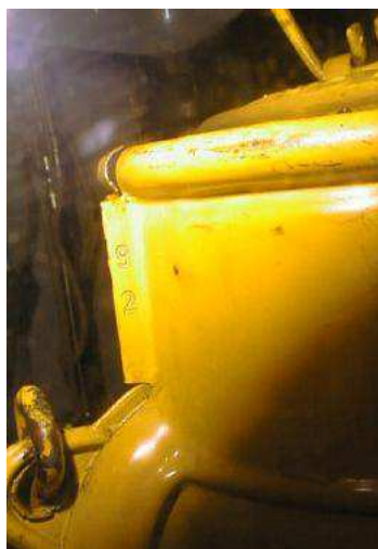
Fig. 8.1: Date of production code 92 (9 over 2) at the folded rim of the Sturmkappe on a Nr.276 "Baby Special" 70-hours traffic guard indicating September 1972 (month over year)
