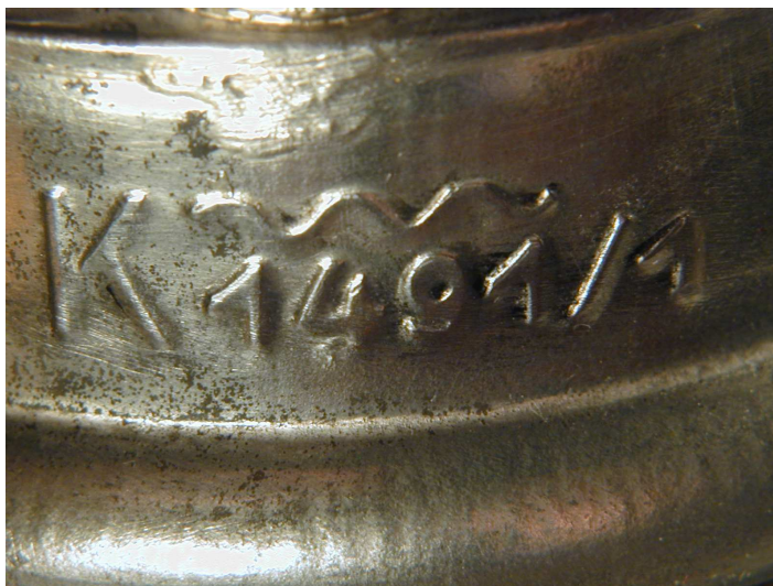
Figure 7: Raised imprint of the test mark of the German "Lichttechnisches Institut Karlsruhe" on the fount of a Nr.175 "Super Baby" with ruby-red globe. This lantern is allowed for use as a rear light for any kind of vehicles.
