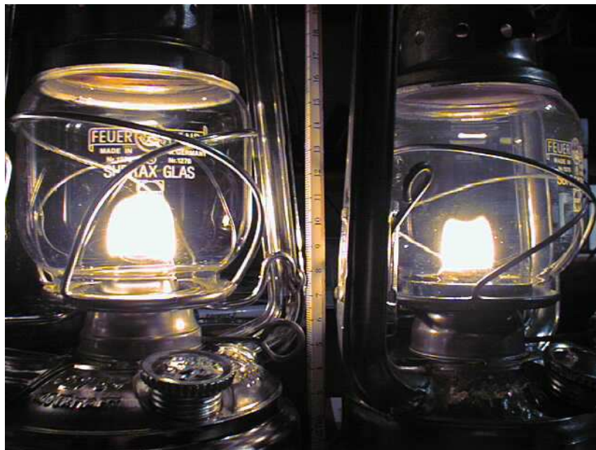
Figure 1: Flames of approximately 5 cd of Gas Oil (Diesel) fueled Storm Lanterns Feuerhand Nr.276 with modified 5'' burners, 13 mm flat wick, and burner plate sieves of different shape.
